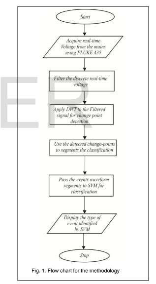
From Fig. 1, the real-time power quality voltage signals are obtained from the mains using Fluke 435. The signals are obtained from household and office appliances such as fans, laptop, television, blender, washing machine and so on. These obtained signals contain various PQ problems such as voltage swell, voltage dip and interruption. The discrete real-time signals obtained are then
