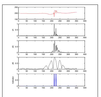
Fig. 3. DWT decomposition of voltage swell for laptop.
